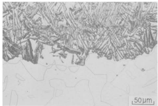
Figure 13 Optical micrograph of the interfacial region of AlN and \gamma matrix for the specimen nitrided in nitrogen at 1000°C for 24 h.
