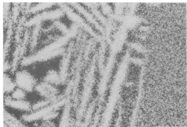
Figure 4 Scanning electron micrograph and X-ray images around the growth front of the needle-like structure as the specimen oxidized in dry air at 1000°C for 48 h: (a) SEM (b) Al K \alpha . (not etched).
